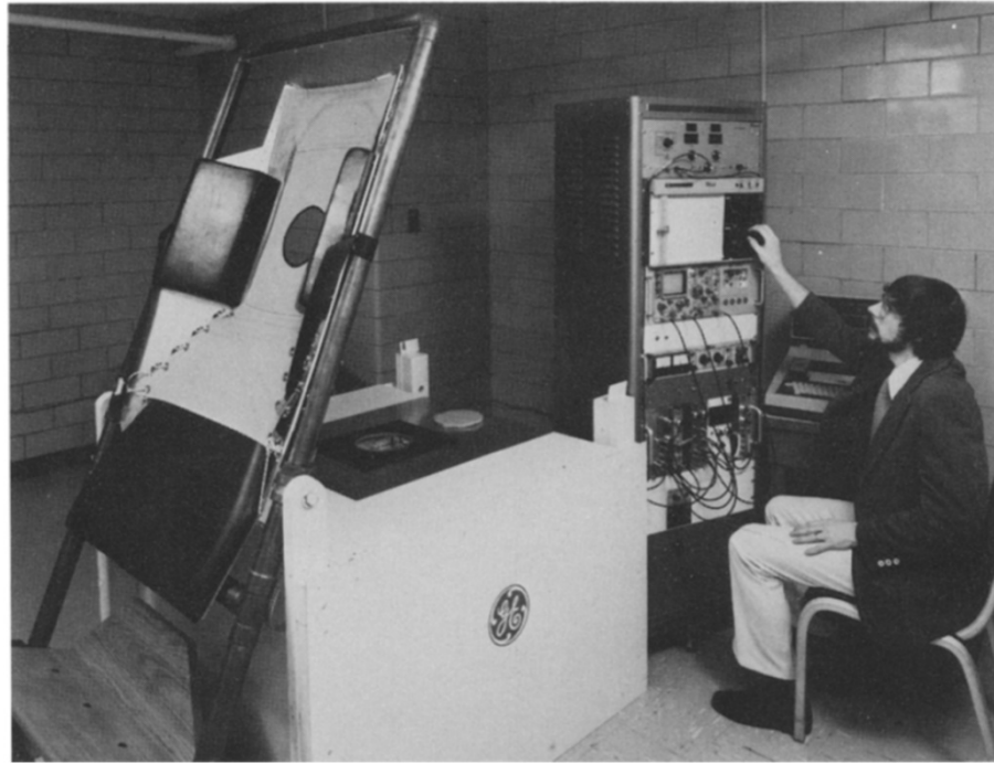
Fig. 2. Photograph of complete scanner table installed at Albany Medical Center. The bed is lowered to a horizontal position with the breast positioned through the hole.
